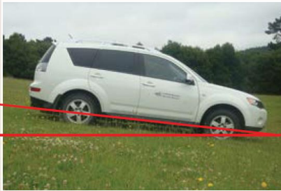
A 6° slope – this is the upper limit of what a traveller should be used on, to manage effluent runoff risks.
